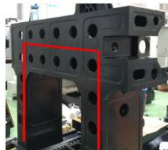
Enlarged and widened "II" shaped beam
